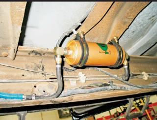
The Fitch Fuel Catalyst was installed along the frame rail inline like a fuel filter. With some applications the Fitch device is installed intank. The correct model unit is determined by the displacement of the engine or the size of the fuel tank. The Fitch device provided a detectable boost in power and also delivered better fuel mileage as promised.
