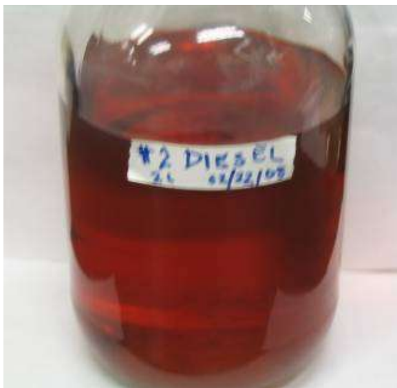
Figure 4. Close view of microbial spoiled diesel DF2 after treatment
