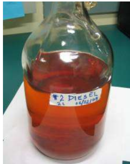
Figure 5. Microbial spoiled diesel DF2 after treatment
