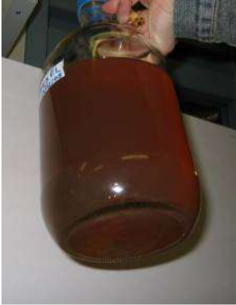
Figure 2. Microbial spoiled diesel #2
