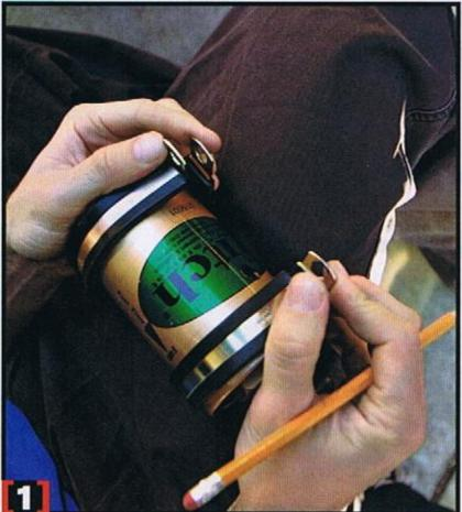
1. To get the system on the move, we mocked up the rubber clamps on the Fitch canister. We then found a location underneath the Nova, near the fuel filter, and marked where we
