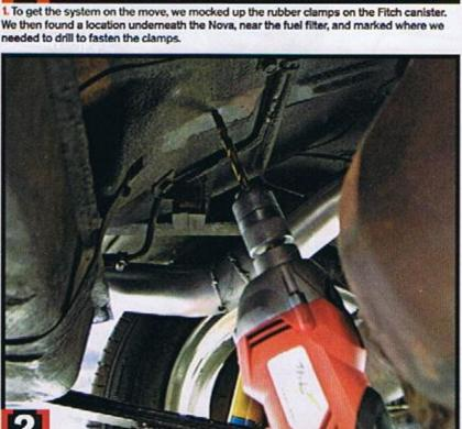
2. Next, we opened the trunk in order to make sure we wouldn't be drilling into anything critical. Using a 29/64-inch drill bit, we drilled two holes, first from the bottom of the car where we had marked with the clamps, and second, for good measure, from the trunk through to the bottom of the car.
