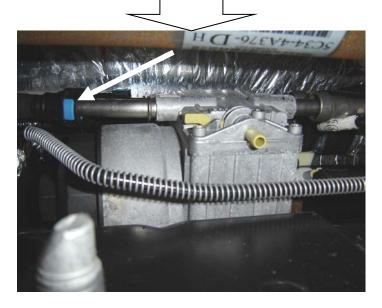
This is a close up view showing the OEM quick connect fitting with the blue locking tap
