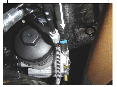
Insert the 90 deg. metal fittings (included in Fitch kit) to each end of the Fitch canister. Mount Fitch Unit in location as shown below.
