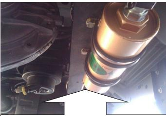
Using the factory holes secure the mounting brackets (included with Fitch kit) around Fitch Fuel Catalyst unit using nuts & bolts for proper installation. Attach each 32" & 20" Fitch fuel hoses to the 90 deg. fitting and run the fuel lines (indicated by arrows above from Fitch over the cross member (indicated with white arrows) for final connection to the OEM female/male quick connects.
